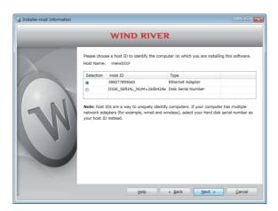
(2) Check the content of "Note" on the window. Select either "Ethernet Adapter" or "Disk Serial Number" for the Host ID and click the Next > button.
